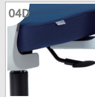
E1-E200 KNEE-TILT Easy KNEE tilt function where the backrest are warped back and seat at the same time, the strength can be adjusted with the lower circular handle, and there is the function of the tilt prevention lever.
